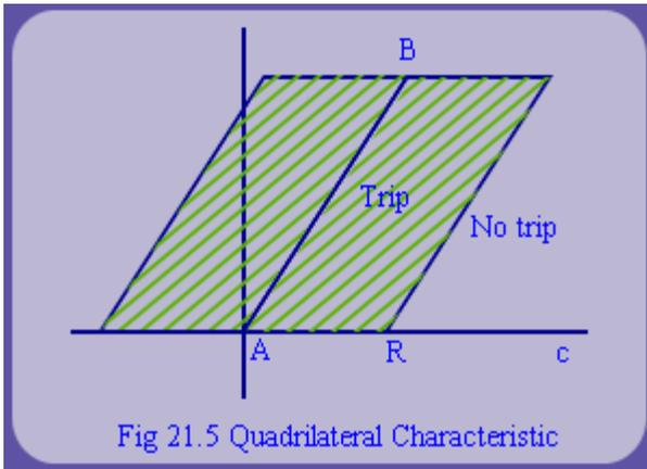
We had so far assumed bolted and unloaded faults. Therefore, there would be errors introduced when the fault has some impedance  $Z_f$ . Hence, the apparent impedance seen by the relay will not exactly lie on transmission line impedance AB. Rather it would lie in a region shown by trapezoid in fig 21.5. Also, note that arcing faults are primarily resistive in nature.
