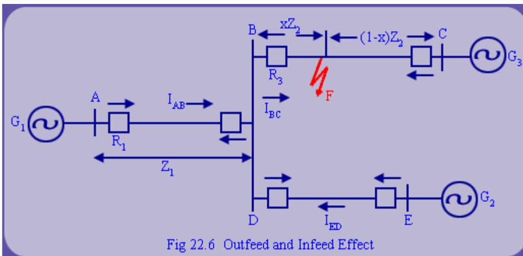
Due to the configuration of generators and loads, we see that  $\vec{I}_{BF} = \vec{I}_{AB} + \vec{I}_{ED}$
