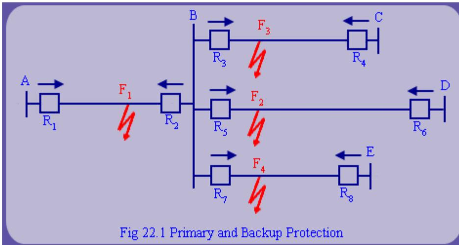
The primary protection should be fast and hence preferably it should be done without any intentional time delay, while back up protection should operate if and only if corresponding primary relay fails. In fig 22.1,  $R_1$  backs operation of relays  $R_3$ ,  $R_5$  and  $R_7$ . Typically, distance relays are provided with multiple zones of protection to meet the stringent selectivity and sensitivity requirements. At least three zones of protection are provided for distance relays.
