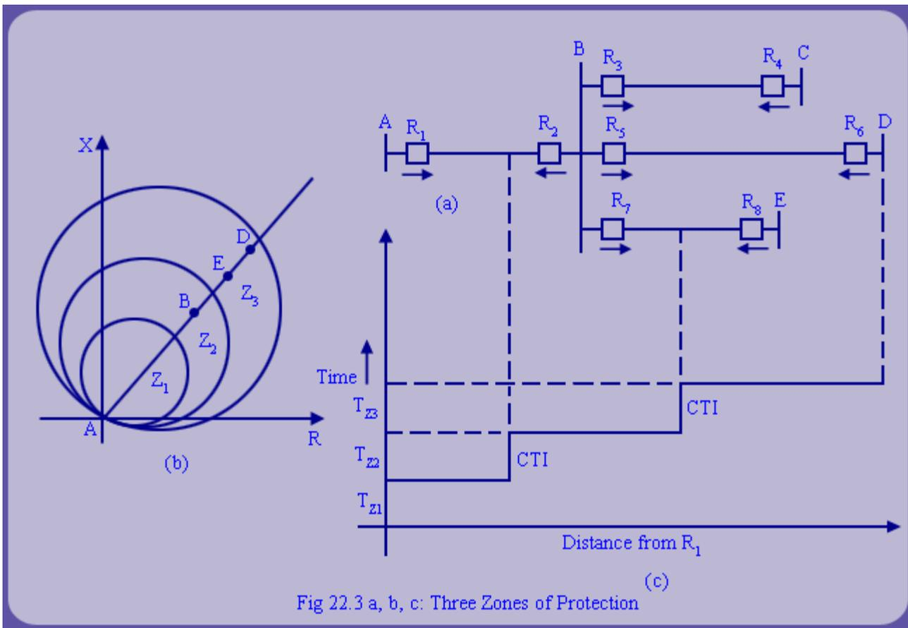
Fig 22.3 a, b, c: Three Zones of Protection
