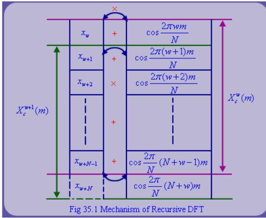
Fig 35.1 Mechanism of Recursive DFT
