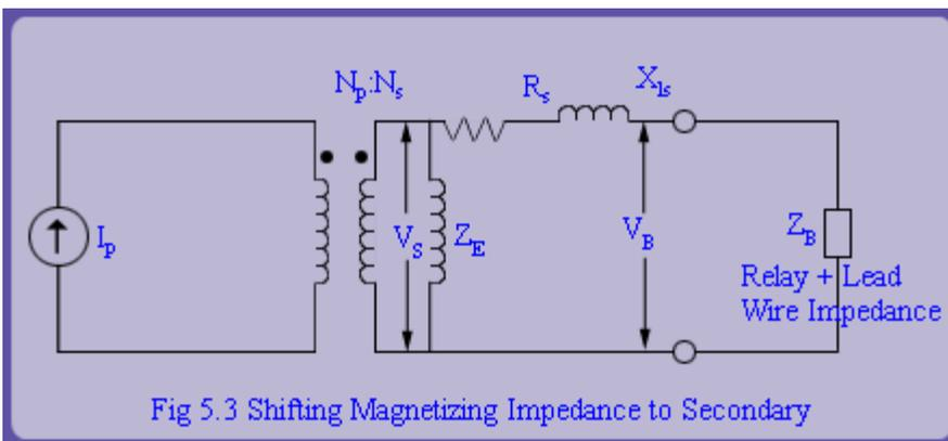
Fig 5.3 Shifting Magnetizing Impedance to Secondary
