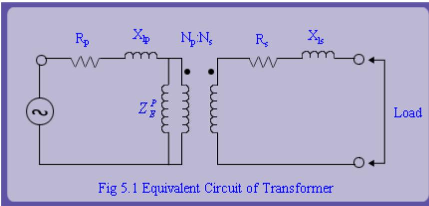
Fig 5.1 Equivalent Circuit of Transformer
