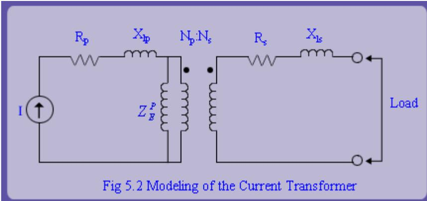
Fig 5.2 Modeling of the Current Transformer
