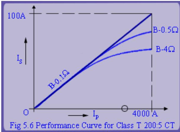
Typically, a class T CT is a wound type CT with one or more primary turns wound on a core. It is associated with high leakage flux in the core. Because of this, the only way to determine its performance is by test. In other words, standardized performance curves cannot be used with this types of CTs.
