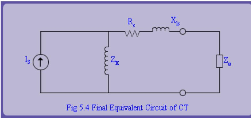
above the knee point, it is more or less obvious that the CT will saturate. During saturation, CT secondary winding cannot replicate the primary current accurately and hence, the performance of the CT deteriorates.
