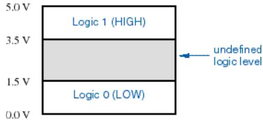
Switching threshold varies with voltage, temp,
