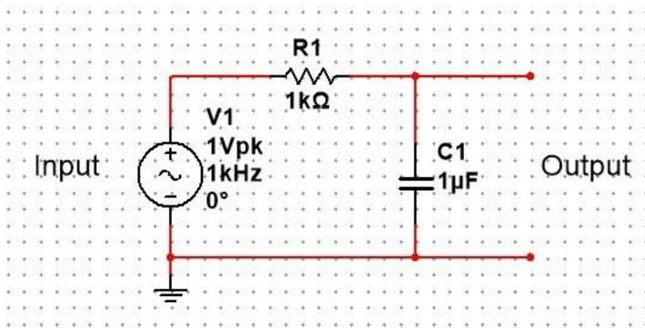
This circuit has a time constant  $t = RC = 10^{-3}$  which corresponds to a 3 dB point at  $1/(2\pi \cdot 10^{-3})$  which is approximately 159 Hz where the voltage gain is 0.7071 and the phase shift is  $45^\circ$ . The gain of this circuit is always less than 1 and the Phase shift never exceeds  $90^\circ$ .
