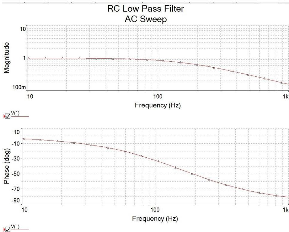
So, if this were the open loop transfer function of a feedback control system, the resulting system would be stable.
