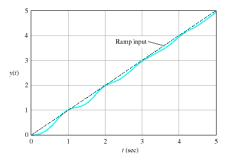
The response to a ramp input for a laser control system
