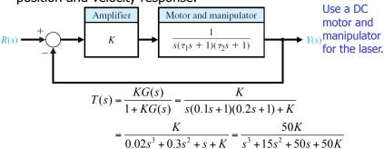
Goal: Find K s.t.  $e_{ss} \le 0.1$  mm for a ramp input r(t) = At where A = 1 mm/s
