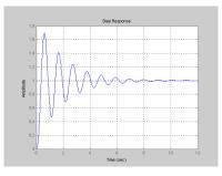
The system response to a step input (highly oscillatory).
