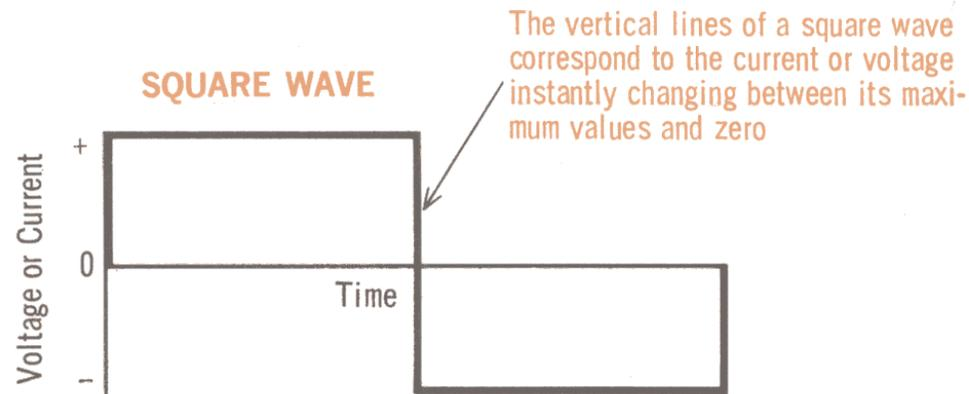
The horizontal lines correspond to steady values of maximum current or voltage
