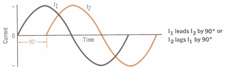
When maximum and minimum points of one voltage or current occur before the corresponding points of another voltage or current, the two are out of phase. When such a phase difference exists, one of the voltages or currents leads, and the other lags
