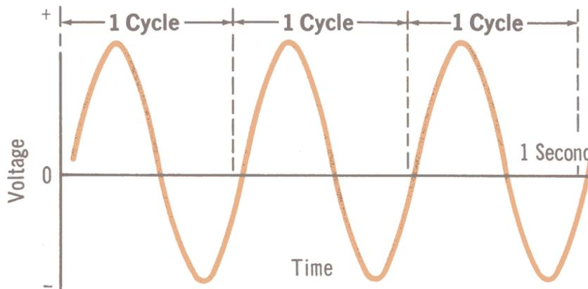
The frequency of a voltage or current is the number of cycles generated each second. The frequency of this voltage is, therefore, 3 Hz
