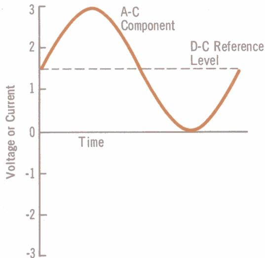
When a d-c voltage or current varies in an a-c way, it does not change direction. However, it fluctuates around the d-c reference level in exactly the same way that ac fluctuates around the zero level
