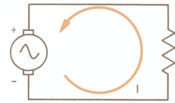
The polarity of a-c power sources changes continuously. Each time the polarity reverses, the circuit current also changes direction
