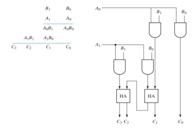
Fig. 4-15 2-Bit by 2-Bit Binary Multiplier
