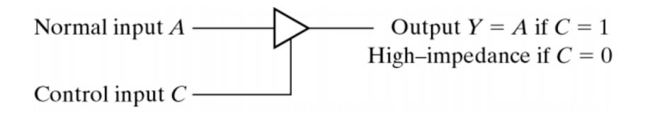
Fig. 4-29 Graphic Symbol for a Three-State Buffer
