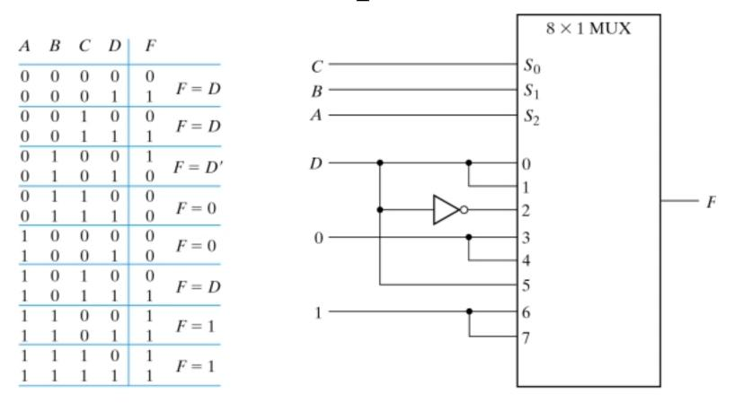
Fig. 4-28 Implementing a 4-Input Function with a Multiplexer
