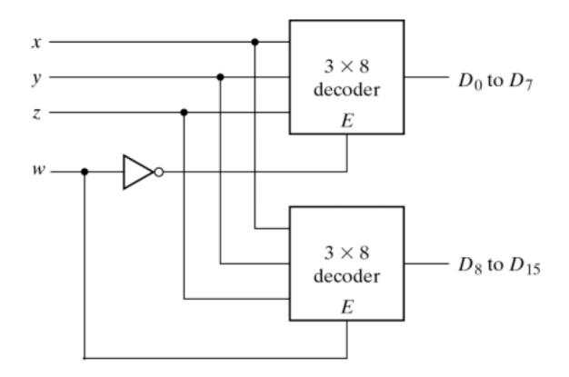
Fig. 4-20 4  $\times$  16 Decoder Constructed with Two 3  $\times$  8 Decoders
