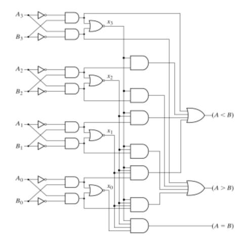
Fig. 4-17 4-Bit Magnitude Comparator
