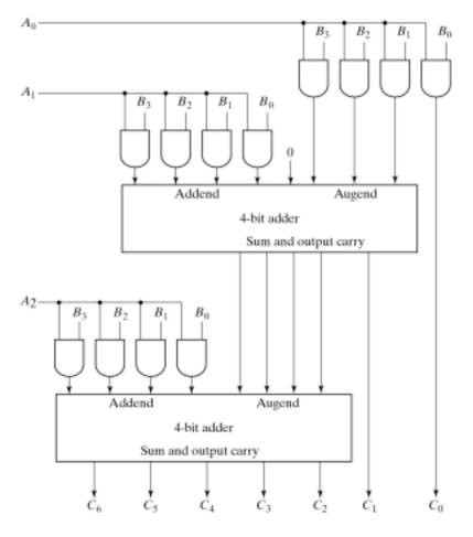
Fig. 4-16 4-Bit by 3-Bit Binary Multiplier
