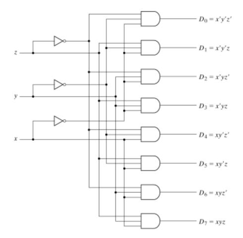
Fig. 4-18 3-to-8-Line Decoder
