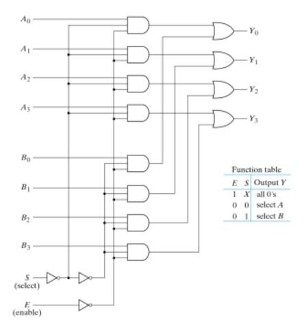
Fig. 4-26 Quadruple 2-to-1-Line Multiplexer
