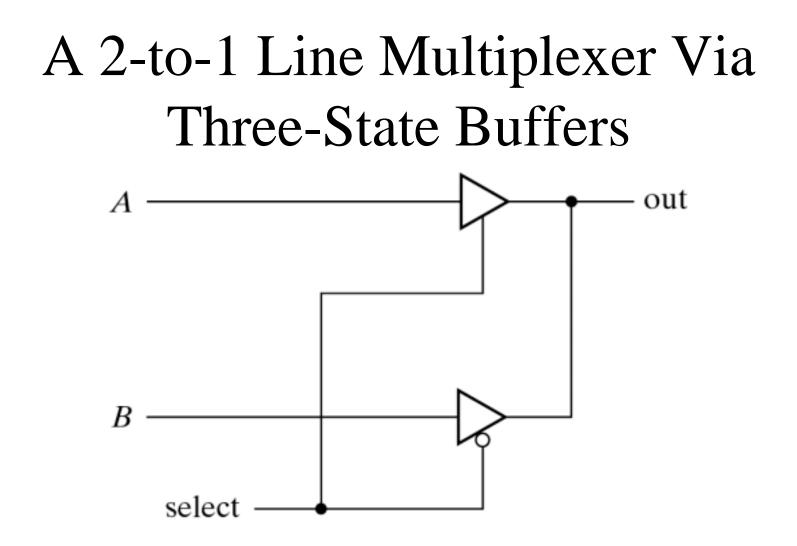
Fig. 4-32 2-to-1-Line Multiplexer with Three-State Buffers
