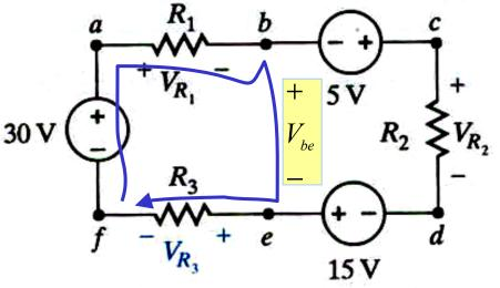
EXAMPLE :  $V_{R1}$ ,  $V_{R3}$  ARE KNOWN DETERMINE THE VOLTAGE  $V_{be}$
