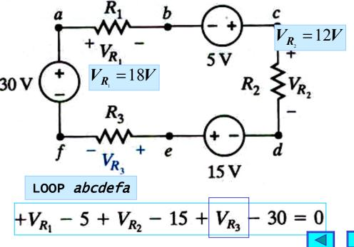
PROBLEM SOLVING TIP: KVL IS USEFUL TO DETERMINE A VOLTAGE - FIND A LOOP INCLUDING THE UNKNOWN VOLTAGE
