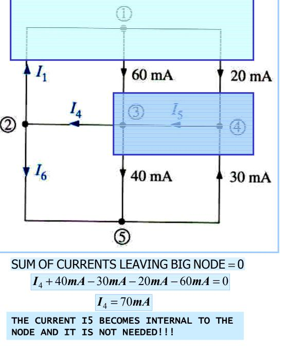
Here we illustrate the use of a more general idea of node. The shaded surface encloses a section of the circuit and can be considered as a BIG node
