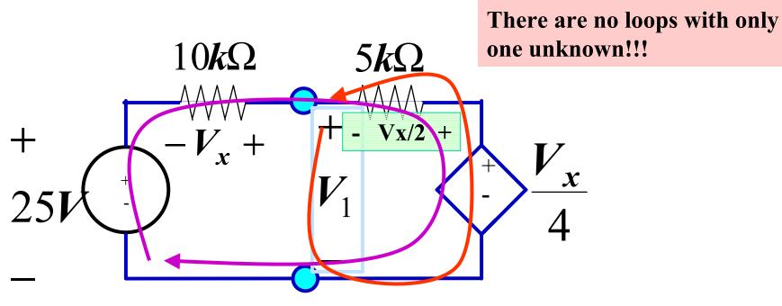
The current through the 5k and 10k resistors is the same. Hence the voltage drop across the 5k is one half of the drop across the 10k!!!
