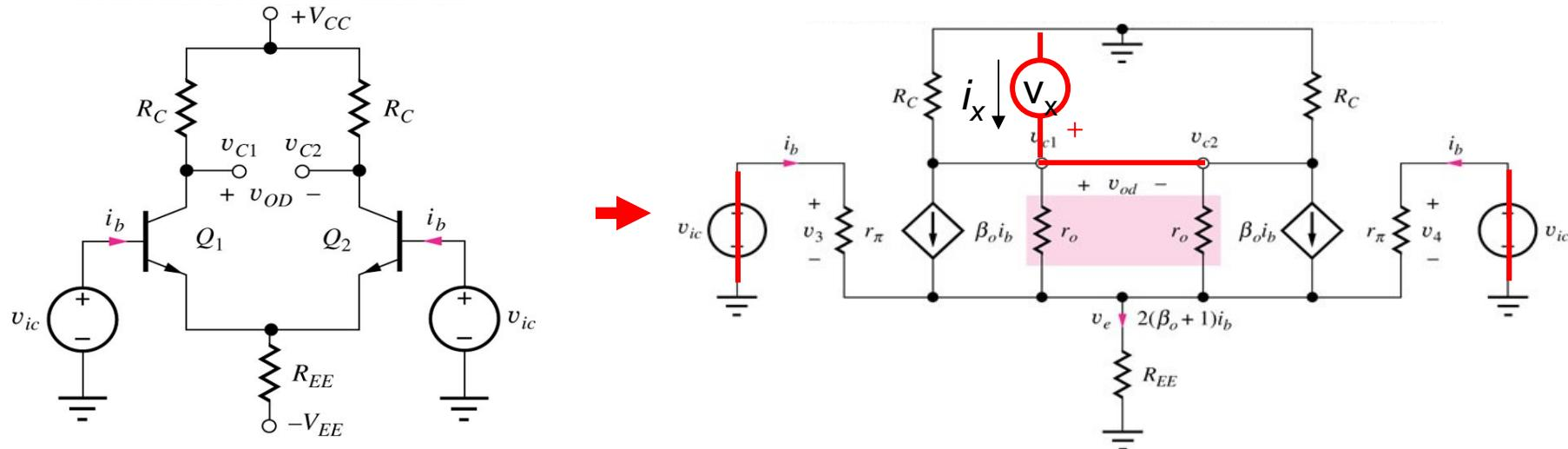
To find CM  $R_{out}$ , tie  $v_{C1}$  and  $v_{C2}$  together and apply a test voltage between  $v_{C1}$  and ground.
