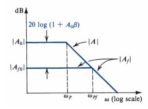
Considering an amplifier with single pole:  $A(s) = \frac{A_0}{1 + s / \omega_P}$
