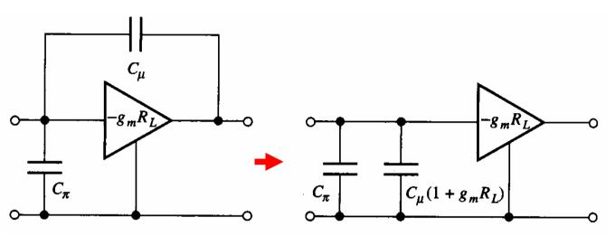
C<sub>µ</sub> is amplified by (1+g<sub>m</sub>R<sub>L</sub>) at the input → Common emitter amplifiers generally have a low upper-cutoff frequency
