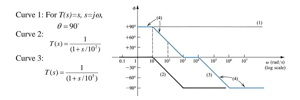
Adding curves (1), (2), and (3), we have curve (4), the Bode plot for the phase response.
