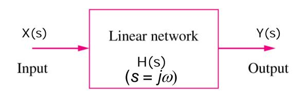
The transfer function of a circuit is the s-domain ratio of an output (voltage or current) to an input (voltage or current) :
