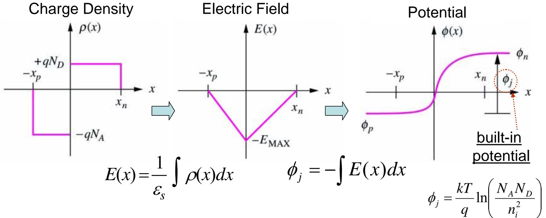
Depletion width is an important device parameter.
