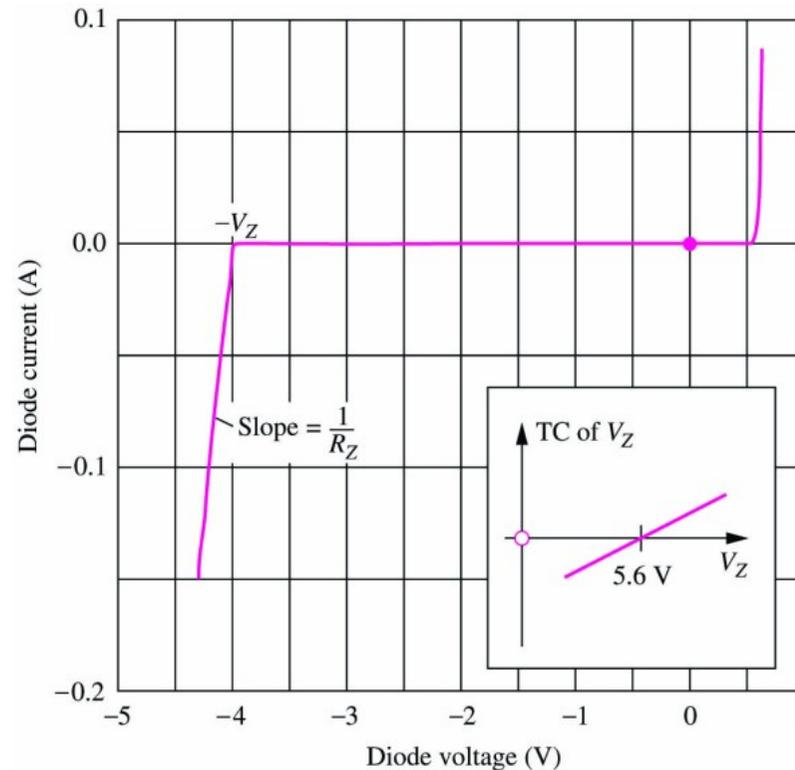
In breakdown, the diode is modeled with a DC voltage source,  $V_Z$ , and a series resistance,  $R_Z$ .  $R_Z$  models the slope of the  $i$ - $v$  characteristic.
