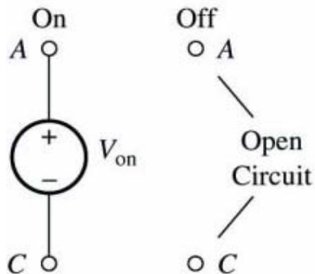
Forward-bias:  $v_D = V_{on}$ ,  $i_D > 0$
