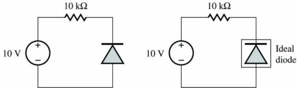
Since source is forcing current backward through diode, assume diode is off. Hence  $I_D = 0$ .
