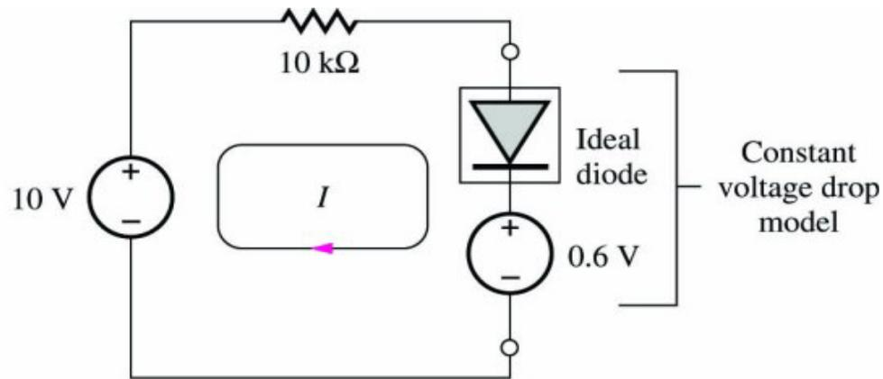
**Analysis:** Since 10V source is forcing positive current through diode, we assume diode is on.
