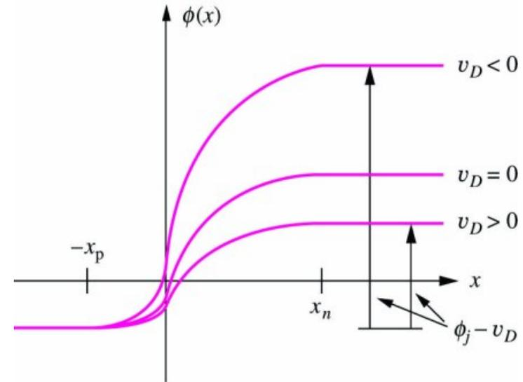
Forward biasing means applying an external voltage  $v_D > 0$ :
