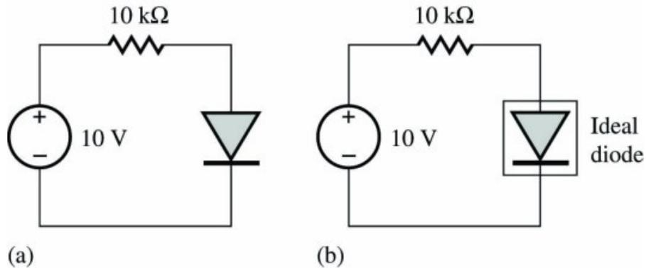
Since source is forcing positive current through diode, assume diode is **on**. So  $V_D=0$ .
