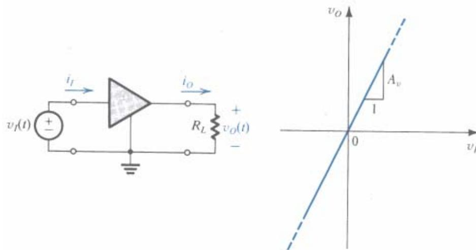
$$\text{Voltage gain } (A_v) \equiv \frac{V_o}{V_i}$$
