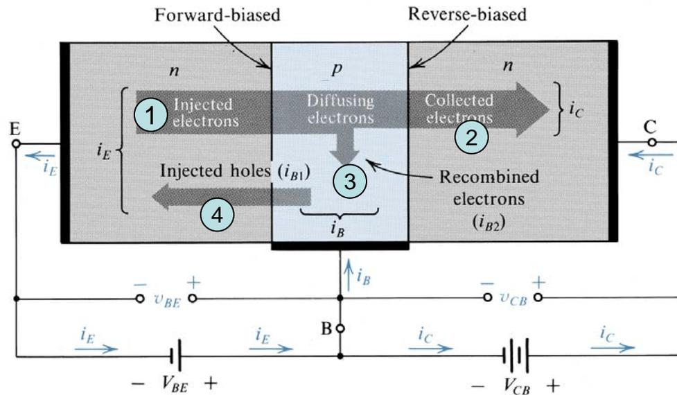
Base current consists of two components:  $i_{B1}$  and  $i_{B2}$ :
