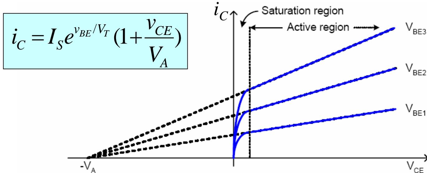
$$i_C = I_S e^{v_{BE}/V_T} \left(1 + \frac{v_{CE}}{V_A}\right)$$
