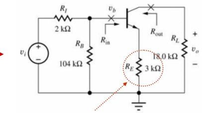
A resistor exists at the emitter of the ac equivalent circuit
