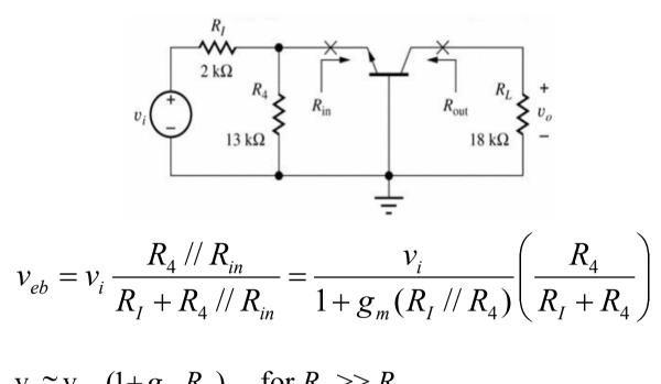
$v_i \cong v_{eb}(1+g_m R_I)$  for  $R_4 >> R_I$ . For small-signal operation,  $|v_b| \le 0.005(1+g_m R_I)V$
