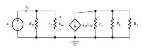
The total resistance looking into the amplifier at coupling capacitor C<sub>1</sub> represents total resistance of the amplifier presented to signal source
