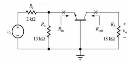
Apply test source to input (E) And use BJT small signal model:
