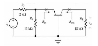
Rout here is equivalent to the Rout of CE amplifier with  $R_E = R_{th}$  and resistance at base equal to zero.
