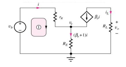
$$R_{in} = \frac{v_b}{i} = r_{\pi} + (\beta + 1)R_E$$
