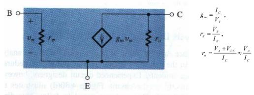
Small signal AC model for BJT (both *npn* and *pnp*) in active mode (T-model):
