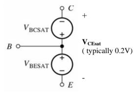
Simplified DC model for *pnp* transistor in active mode:
