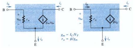
Small signal AC model for BJT (both *npn* and *pnp*) in active mode (Hybrid- $\pi$  model):
