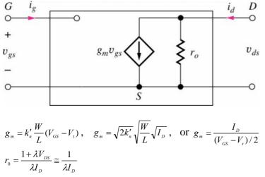
Constraint on  $v_{gs}$  for the small signal model to be valid:  $v_{gs} \ll 2(V_{GS} - V_t)$ , or  $v_{gs} \ll 0.2(V_{GS} - V_t)$ .
