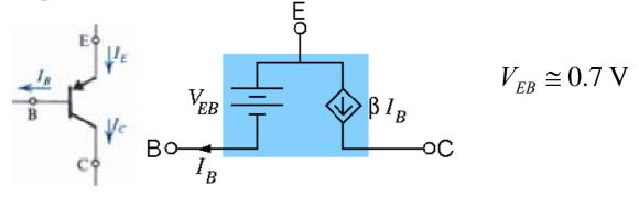
Simplified DC model for *pnp* transistor in saturation mode:
