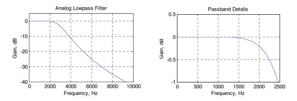
**M4.2** We use N = 3 computed in Problem 4.23 and Fp = 2\*pi\*1500 and Rp = 0.25 and use omega = 0.2\*pi:2\*pi\*10000; to evaluate the frequency points. The gain plot obtained using Program 4\_3 is shown below.
