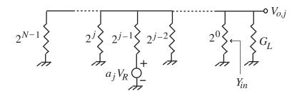
In the above circuit,  $Y_{in}$  is the total conductance seen by the load conductance  $G_L$  which is given by  $Y_{in} = \sum_{i=0}^{N-1} 2^i = 2^N - 1$ . The above circuit can be redrawn as indicated below:
