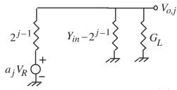
Using the voltage-divider relation we then get  $V_{o,j} = \frac{2^{j-1}}{Y_{in} + G_L} \cdot a_j V_R$ . Using the
