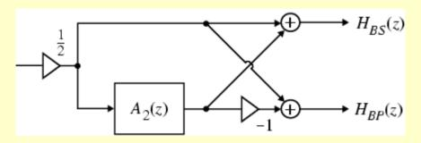
• The 2nd-order allpass filter is realized using a cascaded single-multiplier lattice structure
