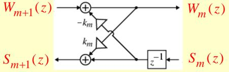
• Its input-output relations are given by  $W_m(z) = W_{m+1}(z) - k_m z^{-1} S_m(z)$   $S_{m+1}(z) = k_m W_m(z) + z^{-1} S_m(z)$
