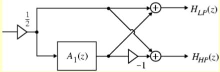
• The 1st-order allpass filter can be realized using any one of the 4 single-multiplier allpass structures described earlier
