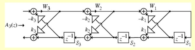
• Objective: Sum the independent signal variables  $Y_1$ ,  $S_1$ ,  $S_2$ , and  $S_3$  with weights  $\{\alpha_i\}$ as shown below to realize the desired numerator  $P_3(z)$
