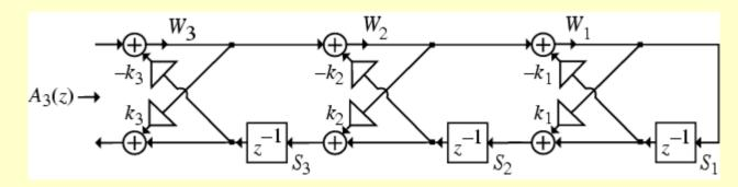
• A typical lattice two-pair here is as shown below
