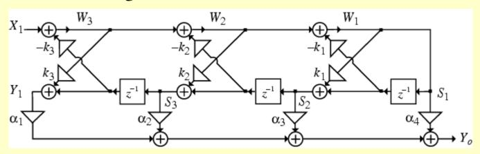
• To this end, we first analyze the cascaded lattice structure realizing and determine the transfer functions  $S_1(z)/X_1(z)$ ,  $S_2(z)/X_1(z)$ , and  $S_3(z)/X_1(z)$
