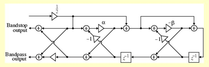
• In the above structure, the multiplier  $\beta$  controls the center frequency and the multiplier  $\alpha$  controls the 3-dB bandwidth
