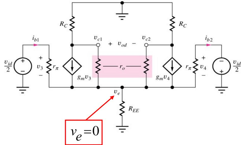
Differential-mode output resistance is the resistance seen between  $V_{C1}$  and  $V_{C2}$ :
