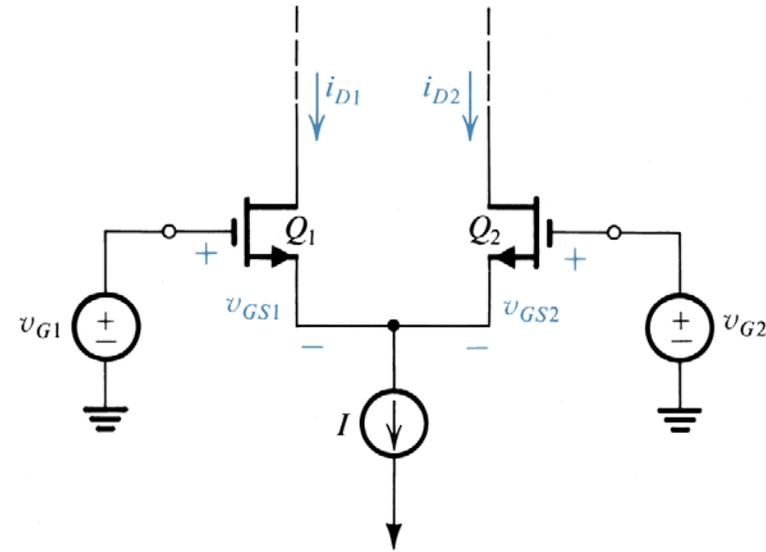
Fig. 6.29 The MOSFET differential pair.
