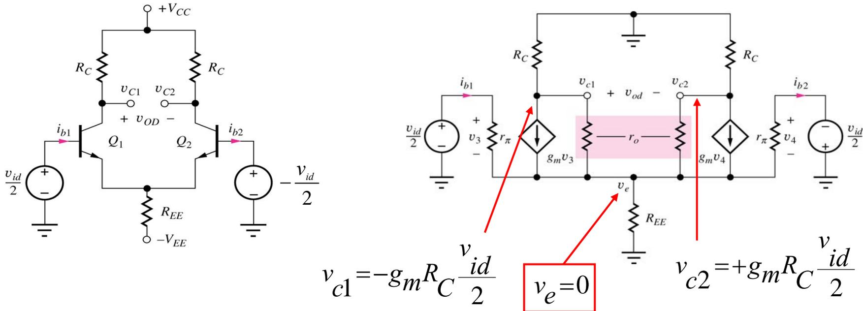
If either  $v_{c1}$  or  $v_{c2}$  is used alone as output, output is said to be **single-ended**.
