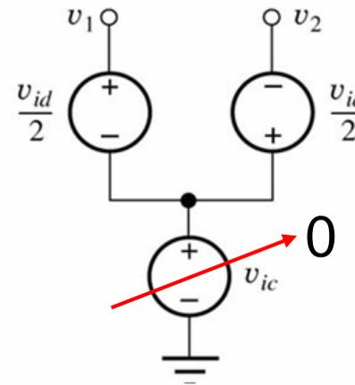
Analyze the circuit by superposition of DM and CM signals
