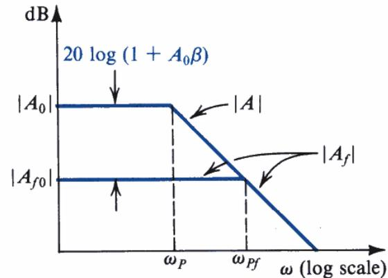
Considering an amplifier with single pole:  $A(s) = \frac{A_0}{1 + s / \omega_p}$
