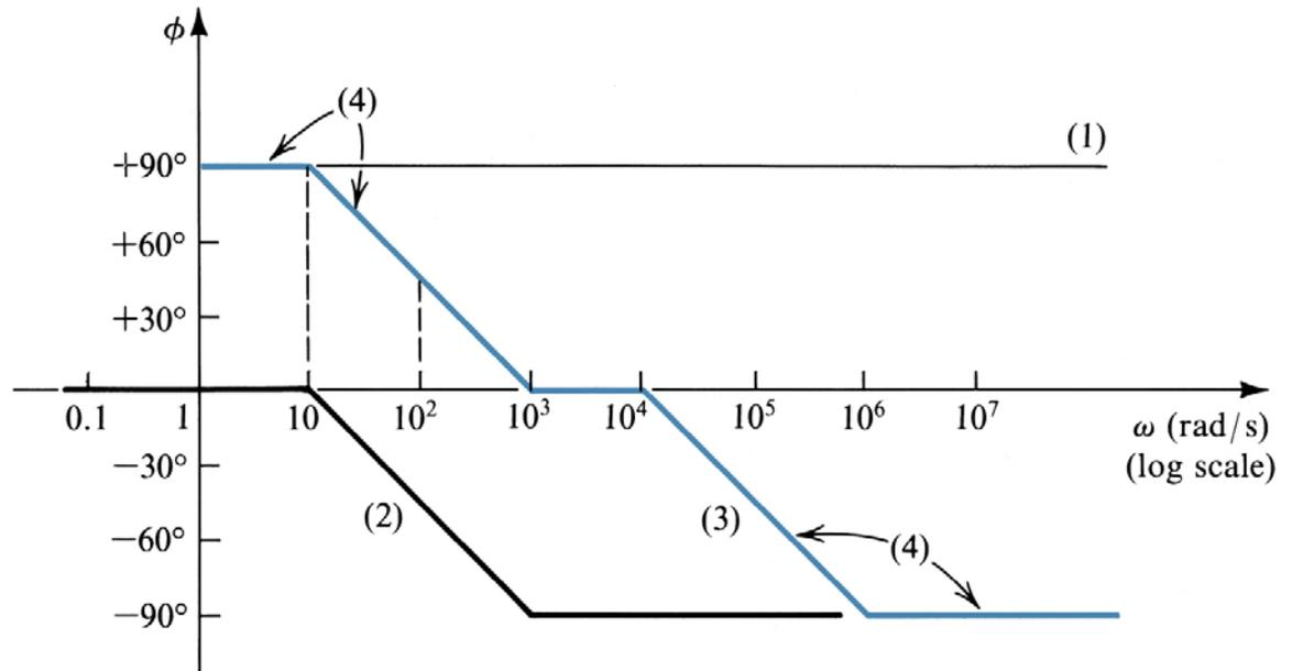
Adding curves (1), (2), and (3), we have curve (4), the Bode plot for the phase response.
