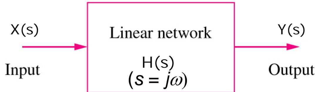
The transfer function of a circuit is the s-domain ratio of an output (voltage or current) to an input (voltage or current) :
