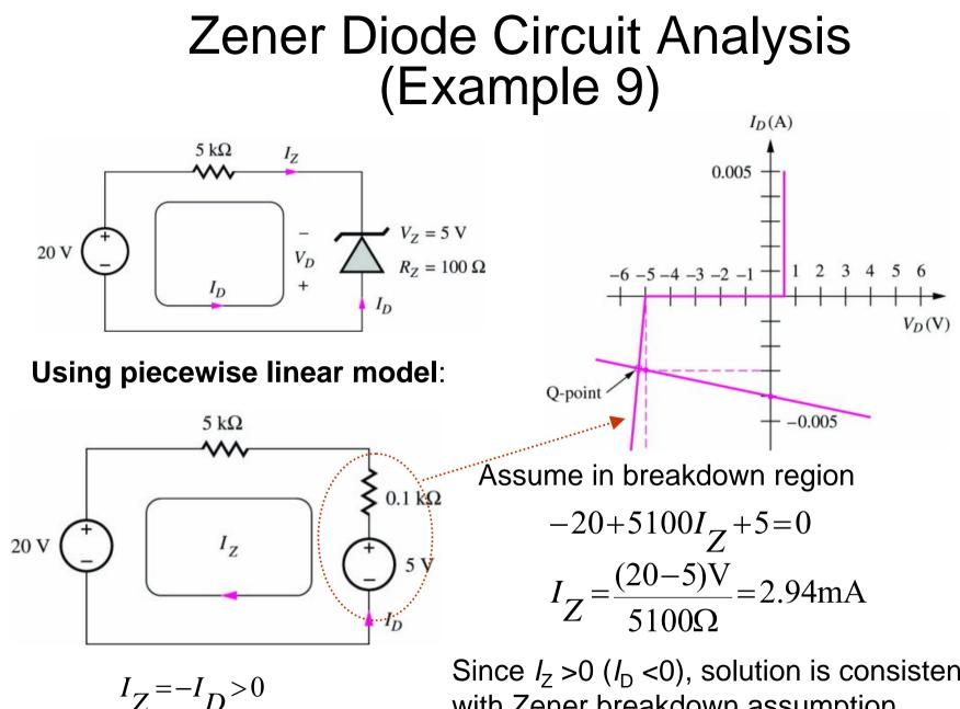
Since  $I_7 > 0$  ( $I_D < 0$ ), solution is consistent with Zener breakdown assumption.
