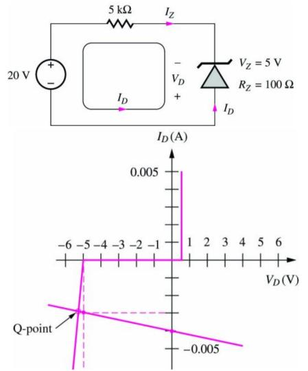
Load-line equation : (KVL along the loop)
