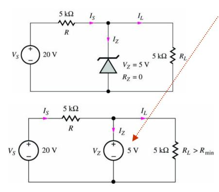
Zener diode keeps voltage across load resistor constant
