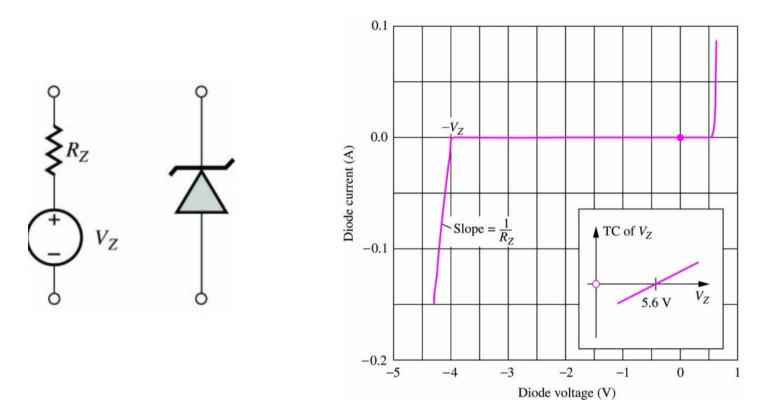
In breakdown, the diode is modeled with a DC voltage source,  $V_Z$ , and a series resistance,  $R_Z$ .  $R_Z$  models the slope of the *i*-*v* characteristic.
