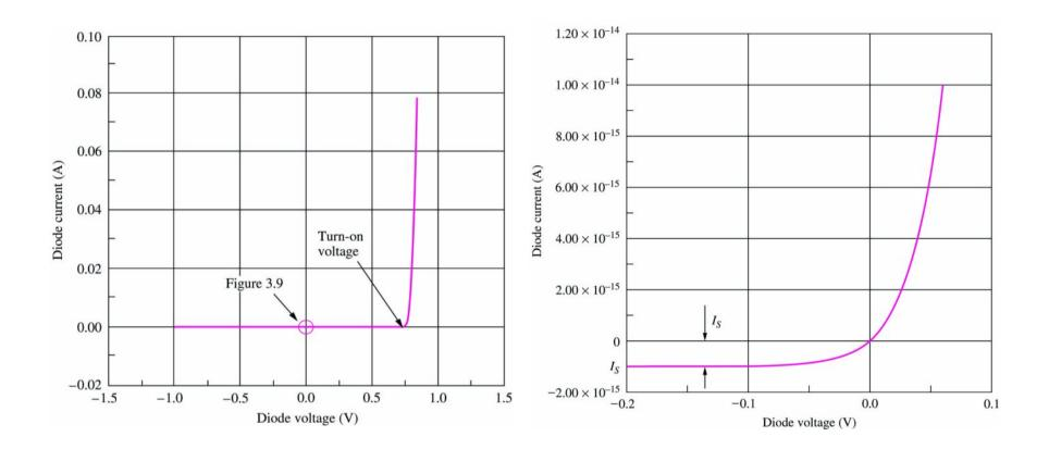
Turn-on voltage marks point of significant current flow.
