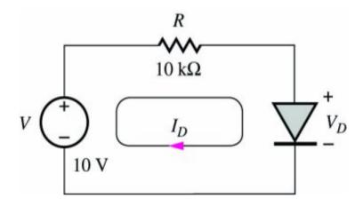
V and R may represent Thevenin equivalent of a more complex 2-terminal network. Full set of equations: 1. Diode equation:
