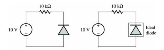
Since source is forcing current backward through diode, assume diode is off. Hence  $I_D = 0$ .
