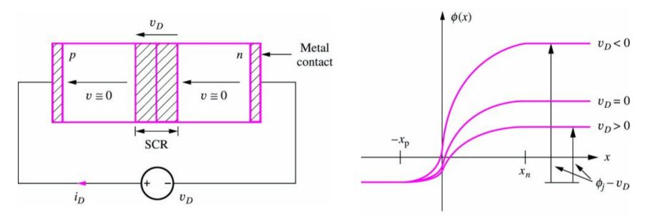
Reverse biasing means applying an external voltage  $v_D < 0$ :
