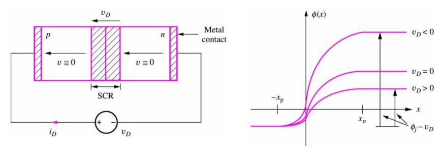
Forward biasing means applying an external voltage  $v_D > 0$ :
