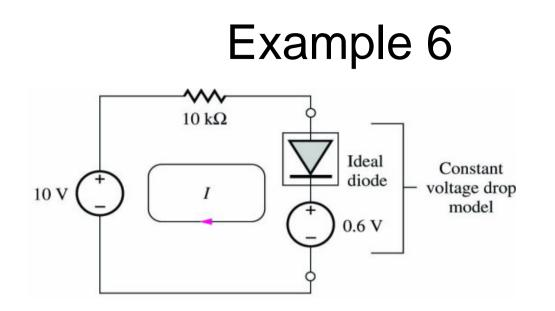
**Analysis:** Since 10V source is forcing positive current through diode, we assume diode is on.
