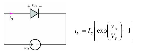
where  $I_S$  = reverse saturation current [A]  $V_D$  = voltage applied to diode [V]  $V_T$  = kT/q = thermal voltage [V] (25 mV at room temp.)
