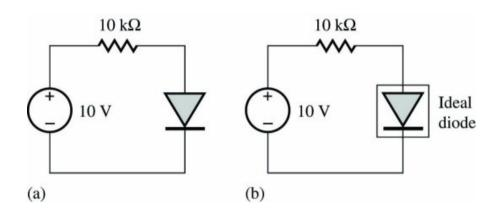
Since source is forcing positive current through diode, assume diode is **on**. So  $V_D=0$ .
