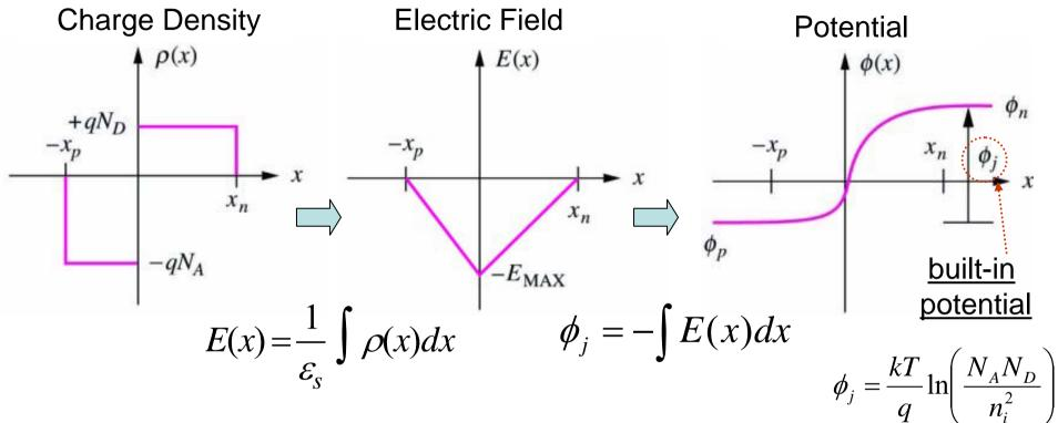
Depletion width is an important device parameter. It can be shown that:
