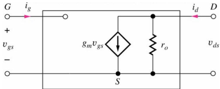
$$g_m = k'_n \frac{W}{L} (V_{GS} - V_t), \quad g_m = \sqrt{2k'_n} \sqrt{\frac{W}{L}} \sqrt{I_D}, \quad \text{or} \quad g_m = \frac{I_D}{(V_{GS} - V_t)/2}$$
