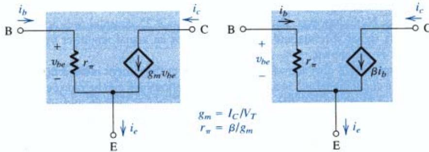
Constraint on  $v_{be}$  for BJT small signal models to be valid:  $v_{be} \ll V_T$  (thermal voltage)
