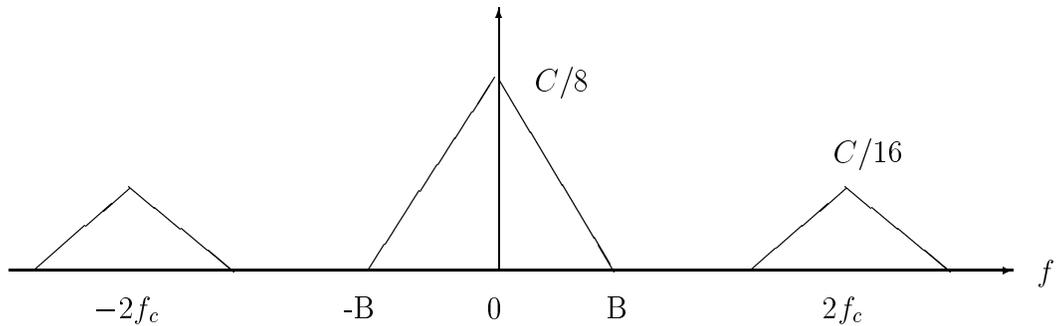
The noise component of the second multiplier output will still be white. Taking LPF to be an ideal low pass filter with bandwidth  $B$  (the message signal bandwidth), the power spectra of the signal and noise components of the low pass filter output then look like
