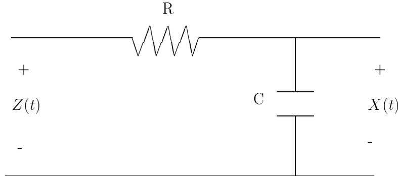
The input voltage  $Z(t)$  is white noise with  $R_Z(\tau) = \delta(\tau)$ . Let us determine the autocorrelation function  $R_X(\tau)$  of the random output voltage  $X(t)$ . From your earlier coursework, you know that the frequency response function of the RC filter is
