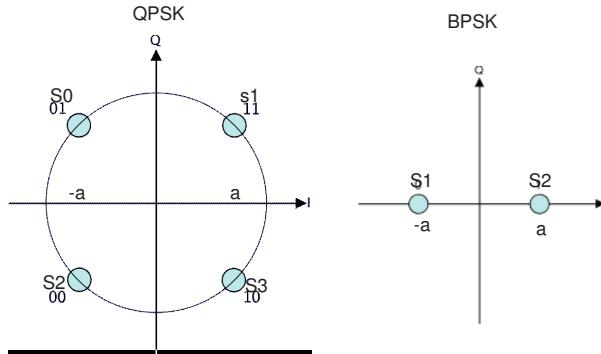
Figure 7.1. BPSK and QPSK modulations
