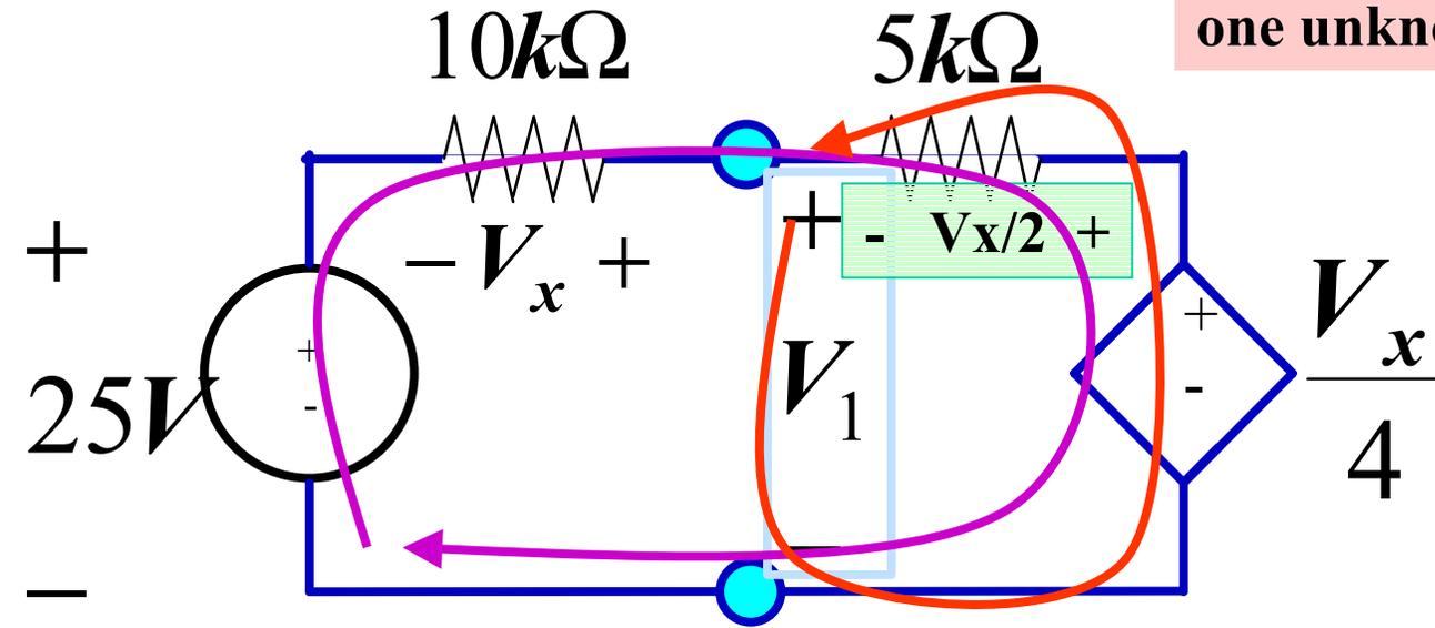
The current through the 5k and 10k resistors is the same. Hence the voltage drop across the 5k is one half of the drop across the 10k!!!
