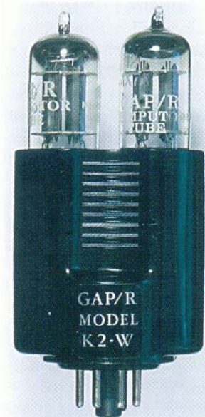
K2-W Op-amp built with Vacuum tube
