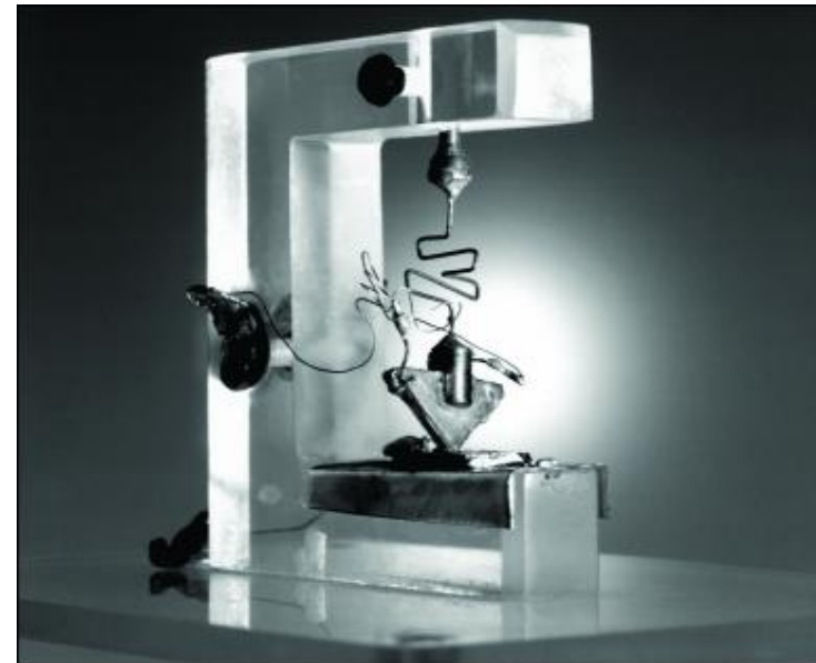
The first germanium bipolar transistor. Roughly 50 years later, electronics account for 10% (4 trillion dollars) of the world GDP.
