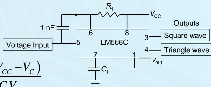
$$f_o = \frac{2.4(V_{CC} - V_C)}{R_1 C_1 V_{CC}}$$
