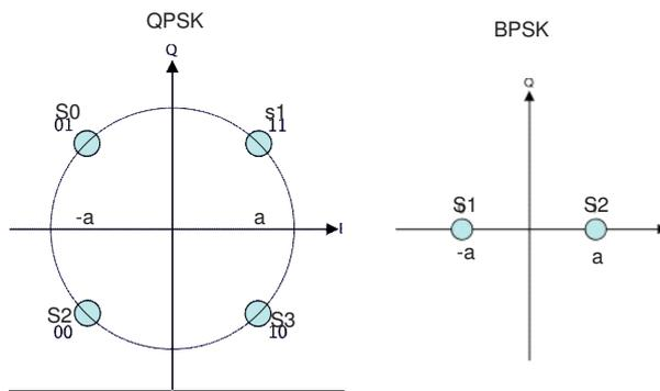
**Figure 7.1.** QPSK and BPSK modulations
