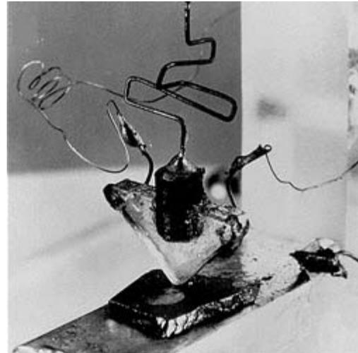
The first transistor looking as crude, perhaps, as the first telephone. Notice how similar the three leads or contacts appear compared to the triode below. The point contact transistor pictured here is now obsolete.
