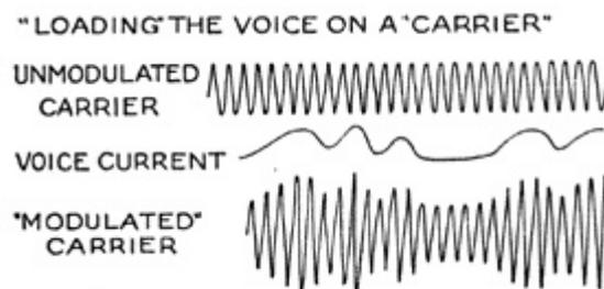
Analog transmission. The unmodulated carrier is simply the electricity your phone operates on, the steady and continuous current your telephone company provides. It carries the conversation. Remember, the telephone is an electrical instrument; electricity works the phone and it carries your voice. When you talk the phone impresses your conversation on the current the telephone company supplies. Conversation causes the current's resistance
