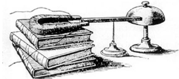
magazine, "a sketch of Henry's primitive telegraph, a dozen years before Morse, reveals the essential components: an electromagnet activated by a distant battery, and a pivoted iron bar that moves to ring a bell."
