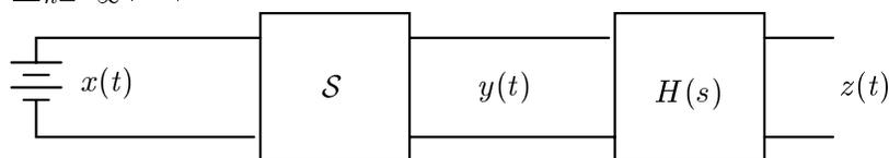
The circuit in the above figure is used for DC to DC conversion. The first stage  $\mathcal{S}$  is a switching system, that periodically alternates between the “ON” state where the output is equal to the input, and the “OFF” state where the output is zero (should be familiar from the midterm...). More precisely, we have  $y(t) = x(t)f(t)$ , where  $f(t)$  is the function in the figure, that alternates between 0 and 1. The constant  $h$  (called the “duty cycle”) satisfies  $0 < h < 1$ .
