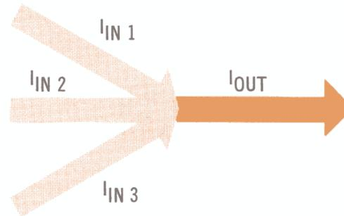
$$I_{IN 1} + I_{IN 2} + I_{IN 3} = I_{OUT}$$
