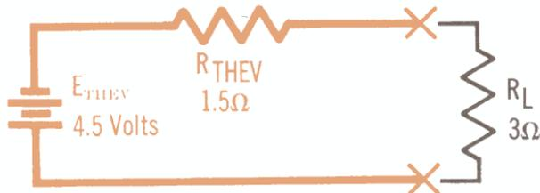
$E_{THEV}$  and  $R_{THEV}$  are connected in series with  $R_L$  to produce Thevenin's equivalent circuit
