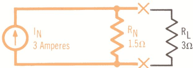
The constant current source,  $I_N$  feeds  $R_N$  and  $R_L$  in parallel to produce Norton's equivalent circuit
