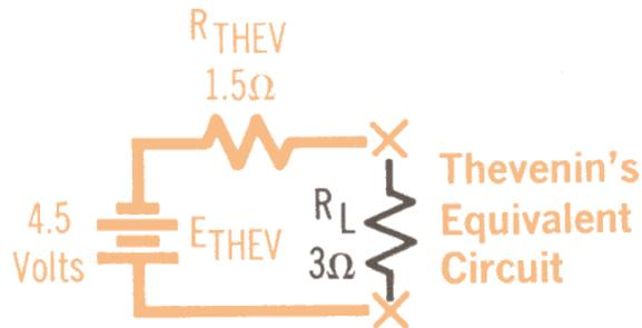
$$\text{Voltmeter reading} = E \left( \frac{R_2}{R_1 + R_2} \right) = 4.5 \text{ Volts} = E_{\text{THEV}}$$
