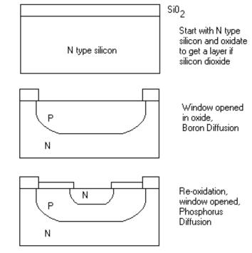
This is followed by another oxidation step and a metalization step (so that you can make contacts for the base, emitter, and collector)
