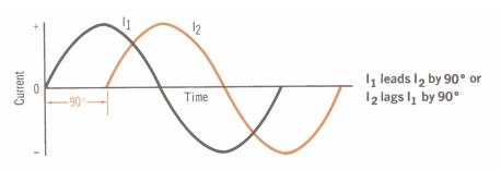
When maximum and minimum points of one voltage or current occur before the corresponding points of another voltage or current, the two are out of phase. When such a phase difference exists, one of the voltages or currents leads, and the other lags
